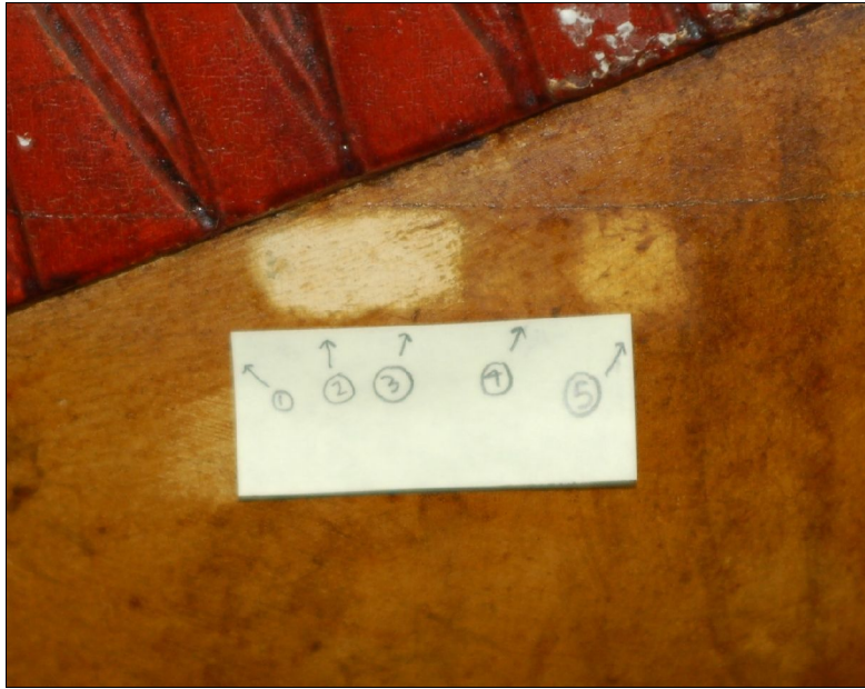
1. Deionized water pH 6 2. Ethanol 3. Acetone 4. 2% Ammonium citrate 5. 5% TEA solution in deionized water buffered to a pH 7.5 with citric acid
